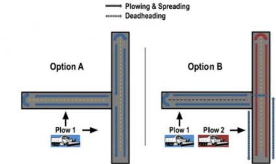
The results of snowplow route optimization can vary depending on an agency's service priorities. The option on the left uses a single plow to achieve lower costs. On the right, the same route can be cleared more quickly with two plows working together. Image courtesy of Clear Roads.
