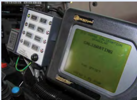
A ground-speed controller in calibration mode.
