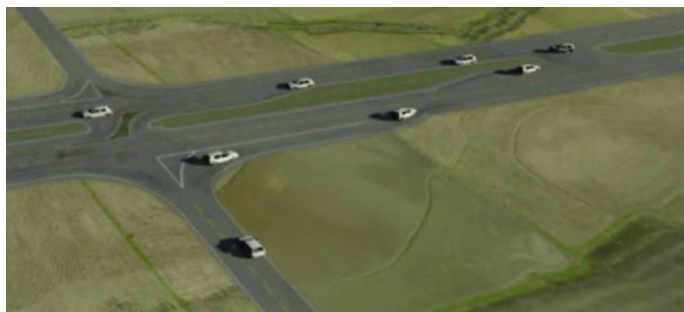
J-turns significantly improve rural highway intersection safety by preventing drivers from directly crossing medians and requiring them instead to make a right turn followed by a U-turn.
