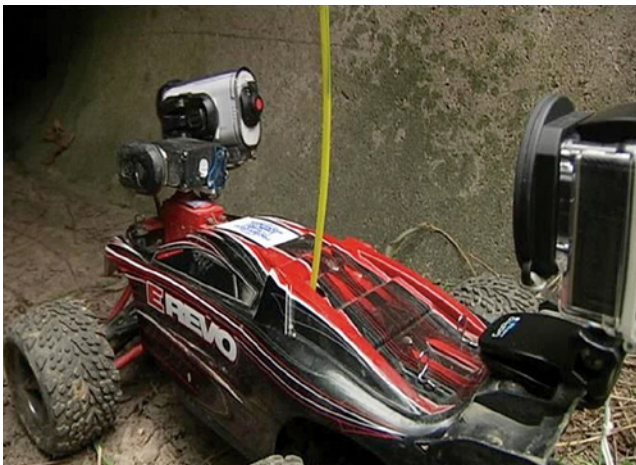
This culvert inspection vehicle, invented by MnDOT staff, is featured in a new handbook on enhanced inspection methods. Photo courtesy of KAAL-TV.
