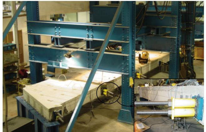
Researchers conducted tests on a half-scale side-by-side box-beam bridge model in order to find a post-tensioning configuration that will minimize longitudinal cracking and significantly extend the performance lives of these bridges.
