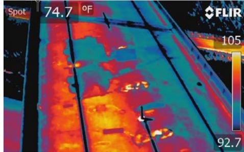
Through thermal imaging (right) that can detect areas of bridge delamination (left), handheld thermographic tools allow for safer, more efficient bridge inspections than traditional methods. This project is providing the field testing, validation and guidelines that MDOT needs to effectively implement this technology.
