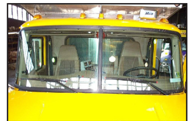
Heated windshield on a Mack truck (photo supplied by Mack).
