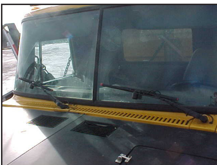
Shaker system installed on Nova Scotia DOT truck (photo from Wiper Shaker Web site).
