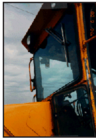
Double-paned windshield developed by Bon Homme County (South Dakota) DOT (photo from LTAP award Web site).
