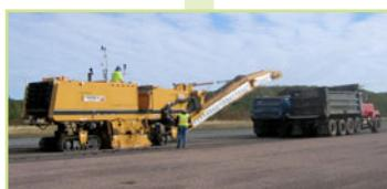
Marquette, Mich. — Prototype water and evacuation system field trials are conducted at an abandoned airport using real-time monitors adapted from NIOSH mining research at critical locations around the machine.
