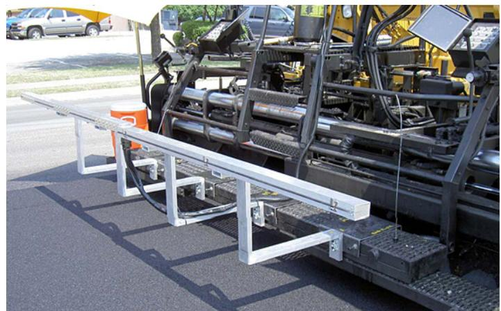
MOBA's paver-mounted PAVE-IR system captures data across the full asphalt mat in real time. (Image courtesy of MOBA)
