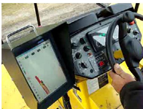
*The pavement might be all black, but the readout of an IC system lets the operator know in living color the number of compaction passes. (Image courtesy of Sakai)*
