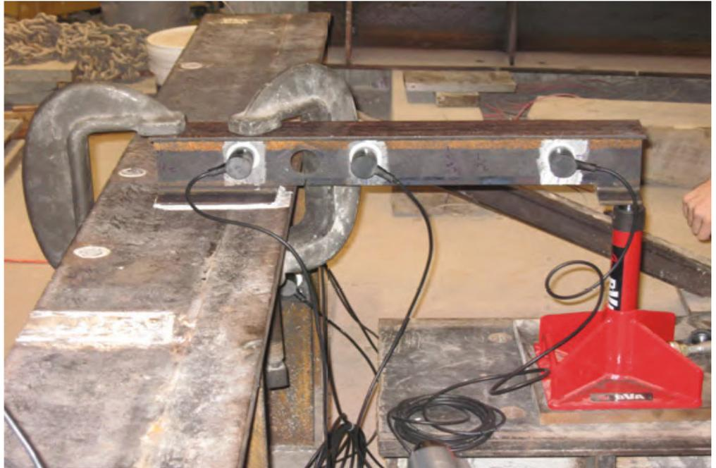
To help distinguish real monitoring events from false alarms, researchers conducted tests to capture acoustic emission data caused by brittle fractures in steel beams using the same bridge health monitoring system currently being used at the Cedar Avenue Bridge.
